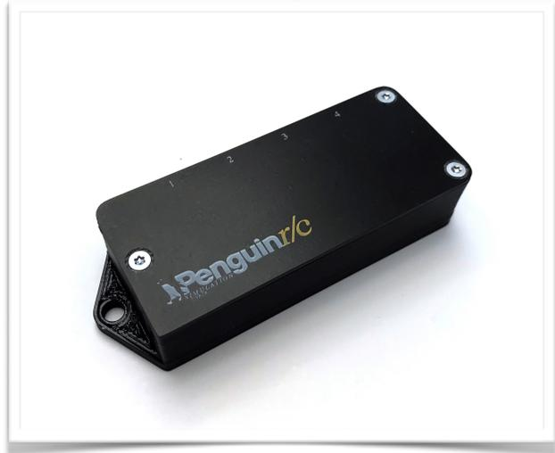
To connect the PSUSB\_28x use the provided cord to connect to any available USB port on your computer. This controller requires no additional software or drivers as it is a standard Windows HID device. The PSUSB\_28x initializes upon being powered up so any setup changes will not take effect until the device is power cycled either by unplugging it or by turning off your computer.
